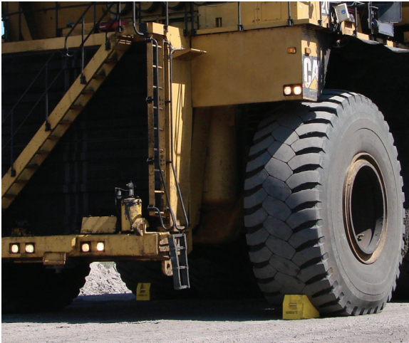
Four Checkers Wheel Chocks, model MC3011 used on CAT 797
