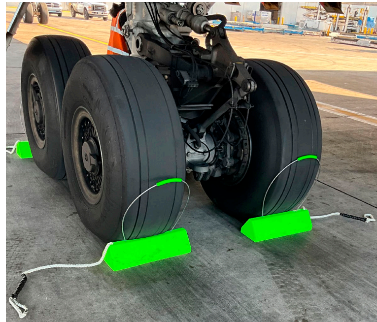
CAC24-QLR-ECH securing 747-400 (cargo) main gear.
