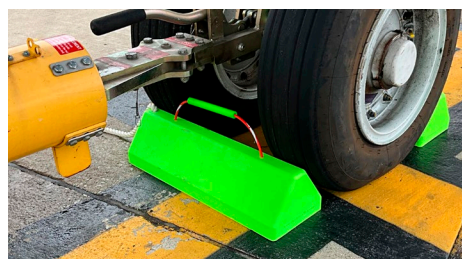
CAC24-QLR securing A320 nose gear.
