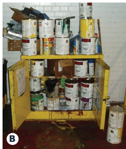
Violation: Flammable items stored on top and outside of cabinet
