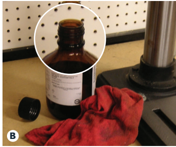
Violation: Open containers are not approved and allow VOCs into the air
