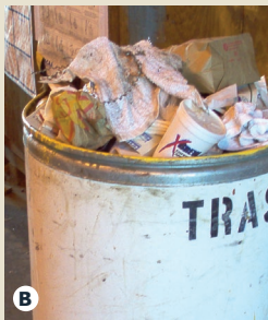
Violation: Fluid soaked wipes in open trash cans
