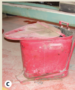
Violation: Inoperable lid, can doesn't close
