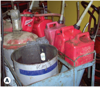
Violation: Not approved metal safety cans
