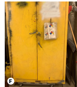
Violation: Cabinets cannot be placed on a wooden pallet
