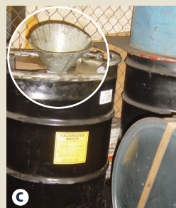
Violation: Not compliant safety funnel or drum lid
