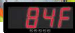
When the temperature reaches user specified setting, the display changes to red.
