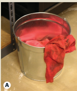
Violation: Fluid soaked rags laying out
