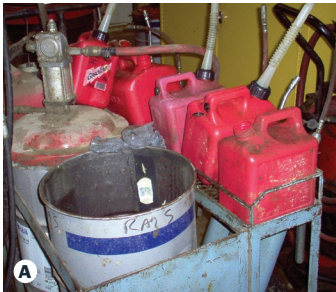
Violation: Not approved metal safety cans
