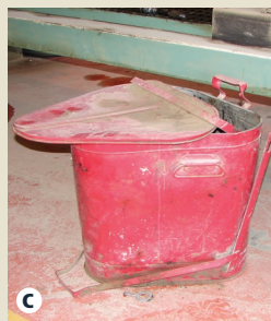
Violation: Inoperable lid, can doesn't close
