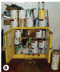
Violation: Flammable items stored on top and outside of cabinet
