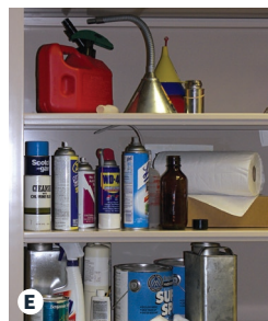
Violation: Flammables on open shelves
